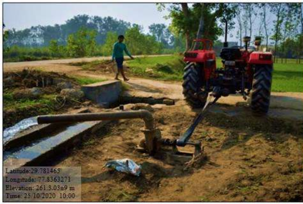
Fig. 4.7: Tractor-operated pump and flow measurement
