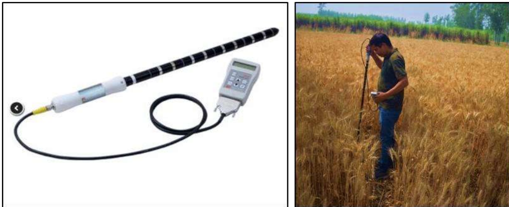
Fig. 6.5: Soil moisture profiler
