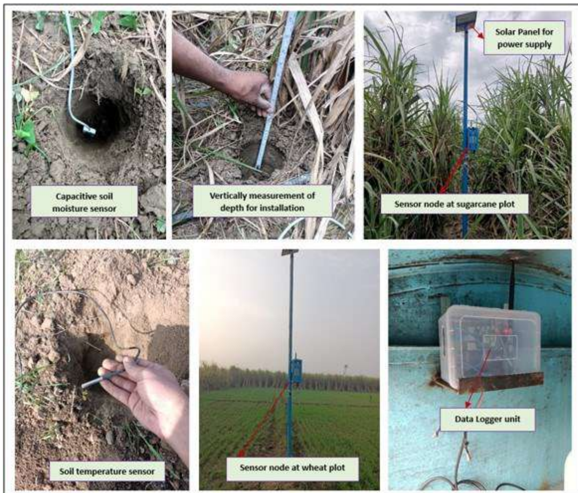
Fig. 5.16: Developed sensors placed with sensor nodes at the irrigation field
